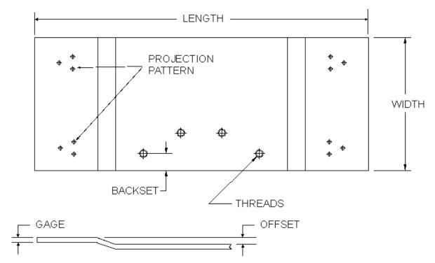
AVAILABLE IN 4 1/2", 5" HOLE PATTERN, THICKNESS 7GA, 1/4", 3/8"(FLAT ONLY), FLAT OR OFFSET, with or without PROJECTIONS
